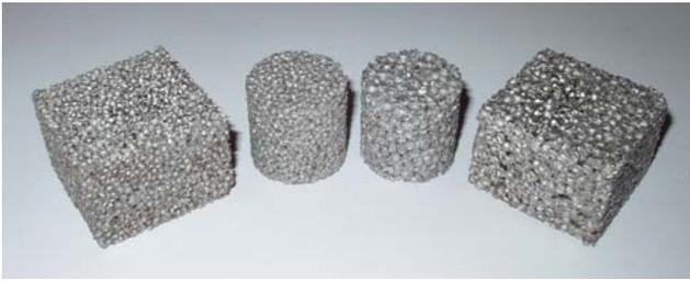
**Fig. 1** Samples of the cellular materials composed of metallic hollow spheres and bonded by sintering technique (MHS)
