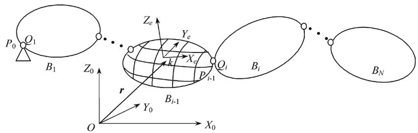
It can be seen that by using absolute nodal coordinate formulation, the centrifugal and Coriolis forces vanish from the equations, and the generalized force vector is constant.
