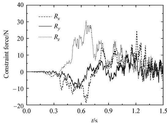
**Fig. 4** Constraint force exerted on  $B_2$  ( $E = 1 \times 10^7 \text{ N/m}^2$ )
