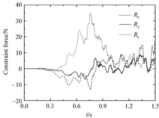
**Fig. 3** Constraint force exerted on  $B_2$  ( $E = 1 \times 10^6 \text{ N/m}^2$ )
