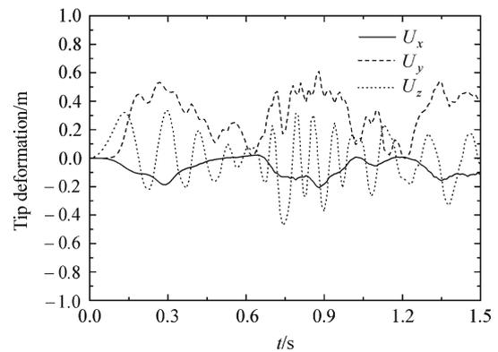
**Fig. 8** Tip deformation of the inner beam ( $E = 1 \times 10^7 \text{ N/m}^2$ )
