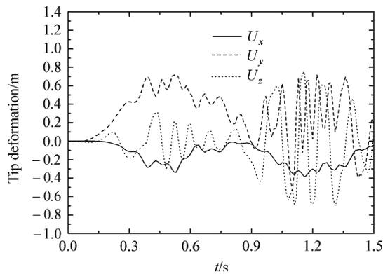
**Fig. 10** Tip deformation of the outer beam ( $E = 1 \times 10^7 \text{ N/m}^2$ )
