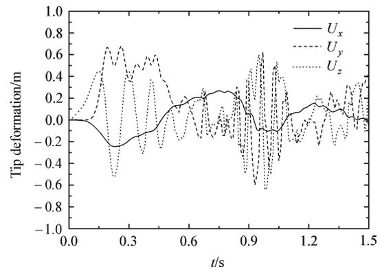
**Fig. 7** Tip deformation of the inner beam ( $E = 1 \times 10^6 \text{ N/m}^2$ )
