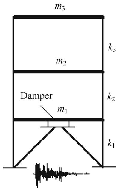
**Fig. 3** Three-story building with a semi-active friction damper at the first floor
