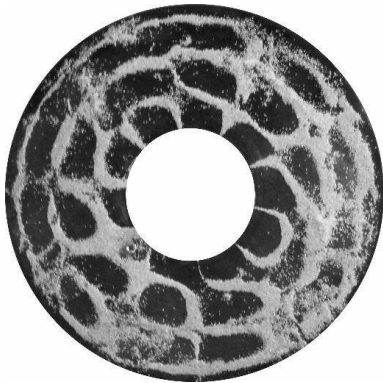
图 1 频率为 2.993 5 kHz 时的实测图 ( m = 5, n = 4 ) Fig. 1 Experiment result while frequency is 2.993 5 kHz ( m = 5, n = 4 )
